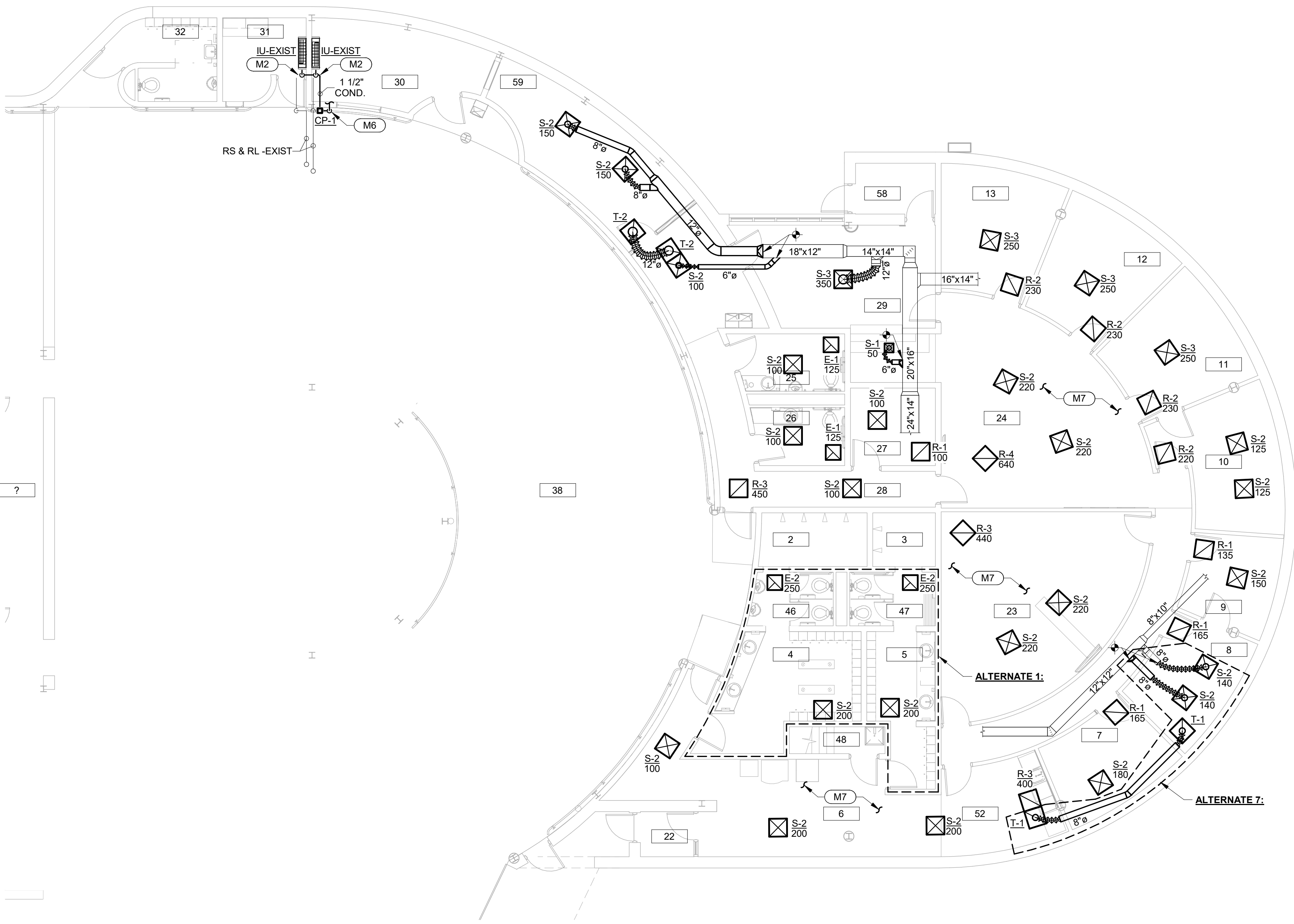
GARAGE EAST FIRST FLOOR HVAC PLAN
