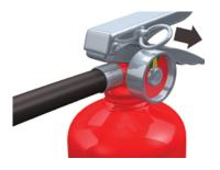
PULL the pin, holding the extinguisher with the nozzle pointing away from you.
