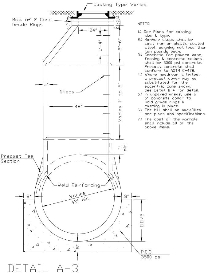
Precast M.H. for 42" Diameter Pipe and Greater Scale 1/2"=1' (Rev. Date 09/01/04)
