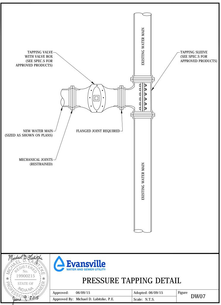
File: J: \ENGINEER\AUTOCAD\Standards\Detail Drawings\Water\DWO7-Pressure Tapping Detail.dwg
