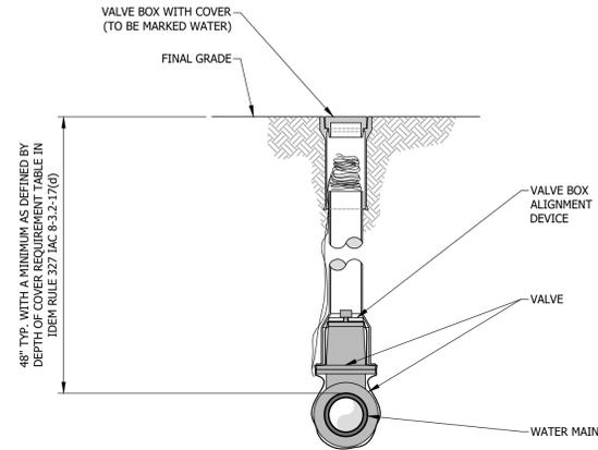
DW03 - GATE VALVE INSTALLATION DETAIL
