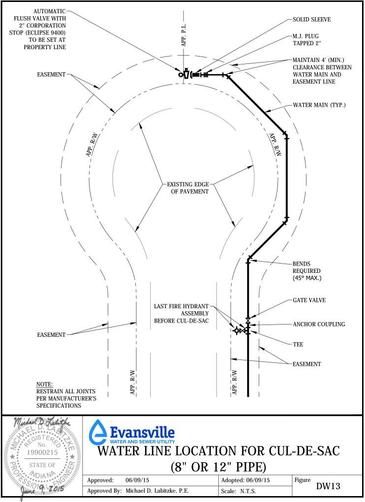
File: J: \ENGINEER\AUTOCAD\Standards\Detail Drawings\Water\DW13-Water Line Location for Cul-De-Sac (8in or 12in pipe).dwg
